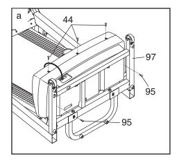
With the help of a second person, carefully raise the Uprights (97) as shown. Carefully pivot the Hood (93) off.
